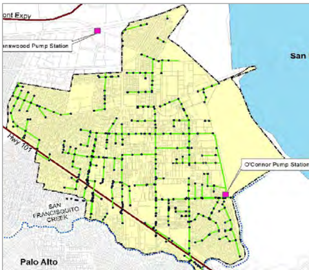
Figure 9-1: Existing Storm Drain System
